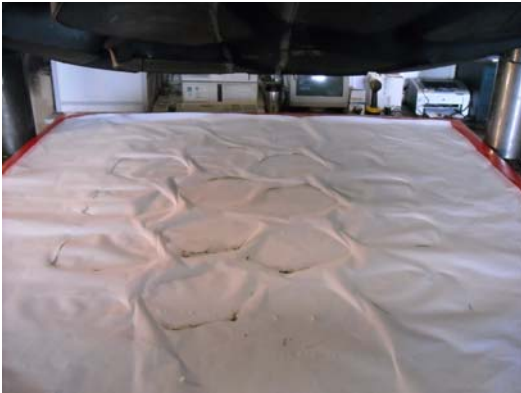
Figure 6: Slip layers become creased over time and need to be replaced.
