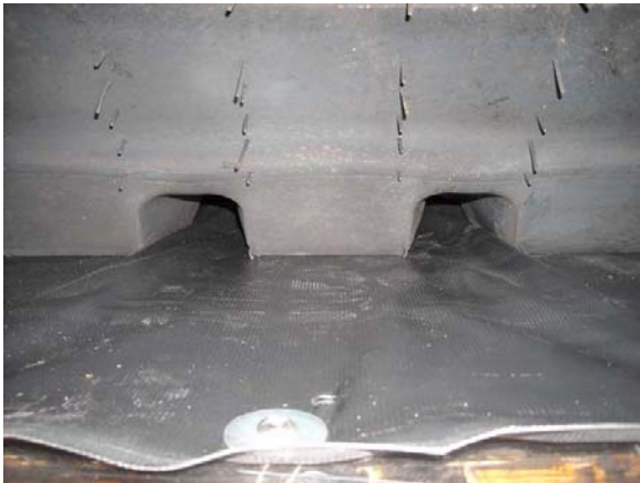
Figure 4: Lug movement across sensor without slip layers will damage the sensor.
