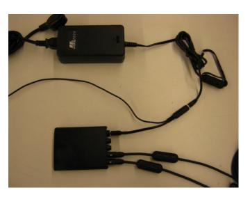
Note: The ground cable is coming off of the left of this picture. The ground cable should be connected using the alligator clip to exposed metal on nearby equipment, or to a known earth ground. For best results, test different grounding locations.
