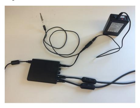
The ground cable should be connected using the alligator clip to exposed metal on nearby equipment, or to a known earth ground. For best results, try different grounding locations.
