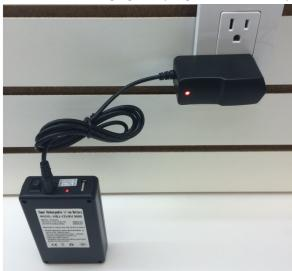
5. Wait for the LED on the charger to change to green (trickle charge) indicating that the battery pack is charged. This may take up to 5 hours.
