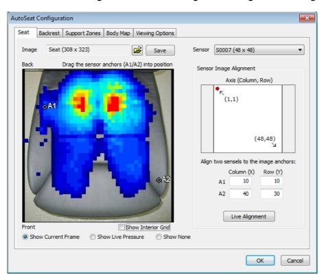
Once a sensor and image are selected, two anchor points (**A1/A2**) may be placed on the image. These are used for properly scaling and aligning the sensor pressure map over the chair image. The anchor points should correspond to two known locations on the seating surface that are covered by the sensing area of the sensor.
