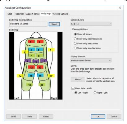
The zone result boxes can be moved from their initial positions. To move a zone box, select and drag it into position using the mouse.
