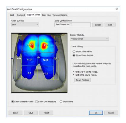
To specify a zone configuration, select Seat or Backrest from the **Chair Surface** drop-list, then press **Select** next to the **Zone Configuration** field to open the **Zone Config Selection** window. (See **Zone Config Selection** below.)
