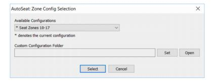
This window shows the available configurations. Select a configuration from the drop-list. The active configuration is demarcated with an asterisk (\*). Configurations created by the user are stored in a custom configuration folder. Select the **Set** button to specify the location of this folder. The **Open** button opens the folder.
