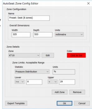
For each zone, the acceptance range of numbers can be entered for all of the available statistics. The relationship operators can also be selected. For example, suppose for Zone KT10's "Pressure Distribution" statistic the following values are selected:
